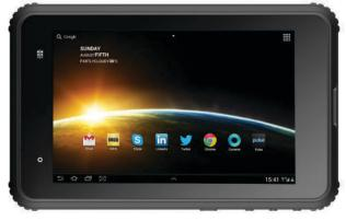
The VT-682 is an 8-inch rugged tablet designed to withstand rough treatment, dust and water ingress, and vibrations associated with in-cab use. Featuring built in GPS for positioning, the tablet also has 4G/LTE mobile connectivity. Running Android 9.0, the VT-682 is ideal for waste management and environmental services applications in challenging environments.
