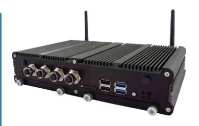
Reliable, fanless vehicle and rail computer with PoE and multiple Mini-PCIe expansion capability. Rugged construction with wide temperature range, shock & vibration resistance and small size provides a powerful computer for many road and rail vehicle applications.
