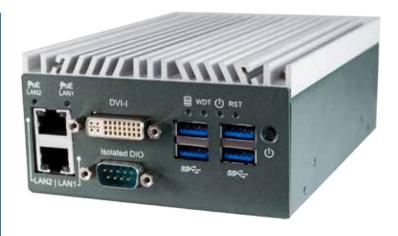
Compact, reliable, powerful, fanless rail computer with multiple I/O capabilities and optional PoE for camera connection. Rugged construction with wide temperature range, shock & vibration resistance and very small size provides a powerful computer for many rail vehicle applications.
