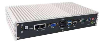
Reliable, powerful fanless rail computer with multiple I/O capabilities. Rugged construction with wide temperature range, shock & vibration resistance and small size provides a powerful computer for many rail vehicle and trackside applications.
