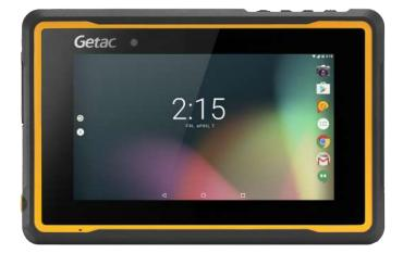
Ideal for mobile workforce and in-vehicle applications in challenging environments. Deploy the Getac ZX70 7-inch rugged Android tablet with confidence knowing it has been tested for extreme conditions and proven by MIL-STD-810G with IP67 ingress protection.
