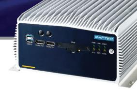
Captec has introduced a range of high reliability, high performance application ready Embedded Fanless Computers (EFC) for a wide variety of industrial applications. The EFC-22 fanless computers have been developed for applications needing robust, high performance computers. They feature third generation Core i processors, remote management, high reliability industrial components, expansion capabilities, wide temperature range and up to 15 years OS life.
